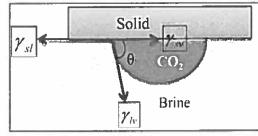
Use the above diagram to derive the Young-Dupré equation relating interfacial tension to contact angle, on an undeformable solid substrate.
