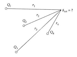
A plan view of a flat area with a piezometer and four fully penetrating wells
