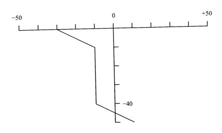
The above potential diagram shows values of the matric potential  $\psi$  (given along the horizontal axis) to vary from -30 to +10 cm with depth below the land surface (given along the vertical axis); values in the above figure are in cm.
