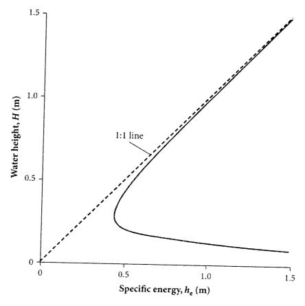
The specific energy diagram for a specific discharge  $q_{\rm w}$  of 0.5 m $^2$  s $^{-1}$
