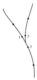
In a stream, the electrical conductivity (EC) is measured in two upstream branches at locations 1 and 2 and downstream at location 3, as shown in the above figure. The EC is linearly related to the salt concentration (mg litre<sup>-1</sup>) of the stream. At location 2 the discharge  $Q_2$  is measured.
