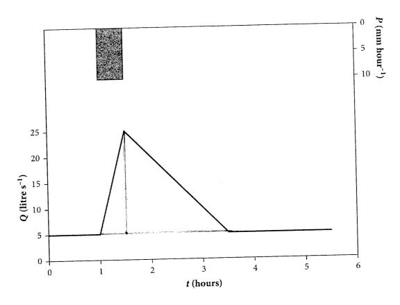
The Kribsbaach drainage basin near Eppeldorf, Luxembourg, has an area of 2 km<sup>2</sup>. The above figure shows a hydrograph with a half hour rainfall event. The discharge on the vertical axis is in litres per second. Time on the horizontal axis is in hours. In the upper part of the above figure the rainfall intensity is given in mm hour<sup>-1</sup>.
