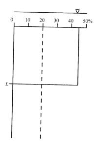
The water level above flat terrain during an experiment with a double ring infiltrometer is kept at 10 mm. The initial moisture content  $\theta_i$  is 20% at all soil depths; the saturated moisture content  $\theta_s$  equals 45%. The saturated hydraulic conductivity K of the soil is 25 mm hour<sup>-1</sup>. During infiltration, the matric potential at the wetting front equals –50 mm. The wetting front is (assumed as) block-shaped: see the above figure (Green and Ampt approach).
