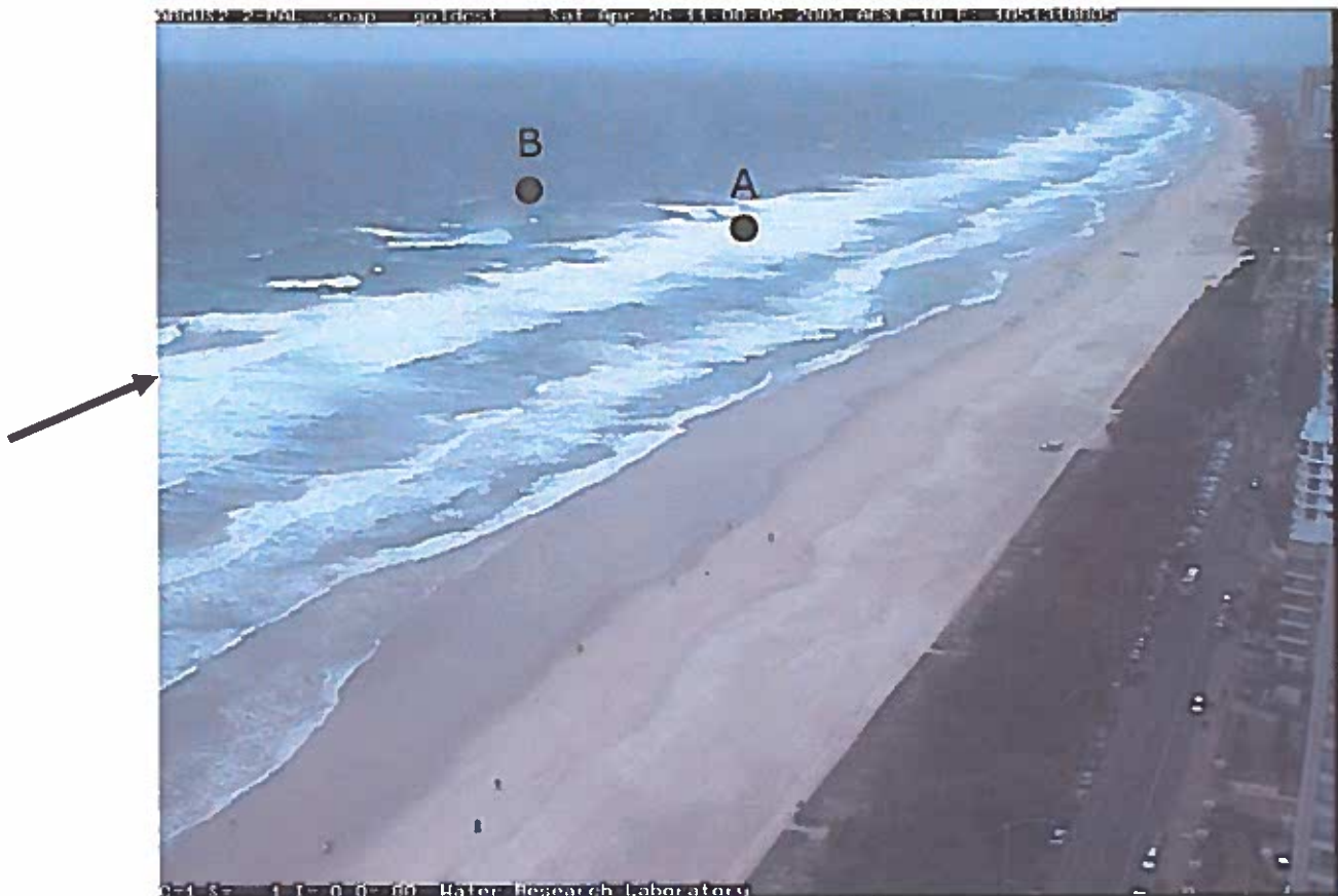
Fig. 2.1: Snapshot (photograph) of a beach during a storm. The arrow points to the alongshore-uniform outer breaker zone above a sandbar (see Fig. 2.2). A and B are locations where cross-shore and alongshore velocities, and sand concentrations were measured at approximately 0.2 m above the sea bed.
