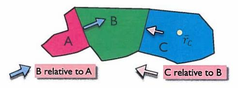
$$\overline{\Delta r}_{CA} = \overline{\Delta r}_{BC} + \overline{\Delta r}_{AB}$$
