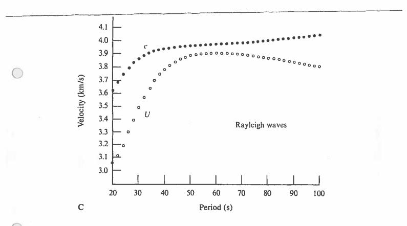
Phase and group velocity of the fundamental-mode Rayleigh waves for the Gutenberg Earth model.
