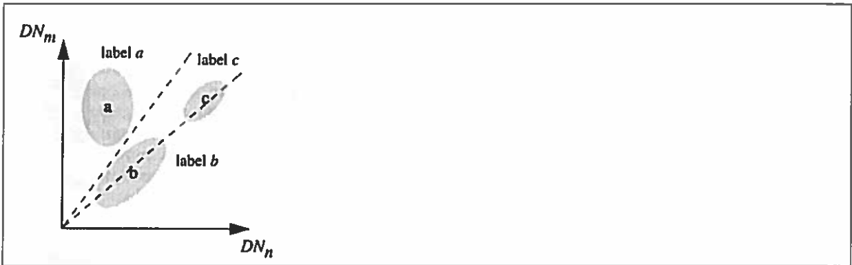
Figure 6.1 Feature space of an image with two spectral bands n and m.
