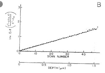
The above experiments were carried out in capsules under high pressure and temperature.  $CO_2$  doped with the isotope  $^{13}C$  at constant concentration  $c_1$ , was used as a fluid in contact with the crystal surface during the experiment and the diffusive process modelled by assuming a semi-infinite medium with constant surface concentration. The solution of the "diffusion equation" came from Crank
