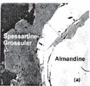
A natural diffusion couple has been produced by an overgrowth of a Spessartine-Grossular garnet upon a core of Almandine garnet (see Figure-a). The overgrowth was formed during a contact metamorphic event and has been subjected to a later, high temperature, prolonged metamorphism to produce a diffusion of Fe, Mn, and Ca between the overgrowth and core (see Figure-b). The Spessartine-Grossular overgrowth contains
