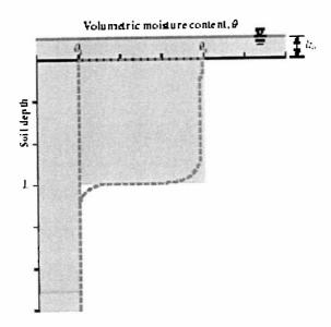
The water level above flat terrain during an experiment with a double ring infiltrometer is 20 mm. The saturated hydraulic conductivity K of the soil is 20 mm hour<sup>-1</sup>. The matric potential at the wetting front equals -60 mm. The initial moisture content  $\theta_i$  is 20% and the effective porosity  $n_e$  equals 45%. Infiltration is (simplified as) block-shaped: see the above figure (Green and Ampt's approach).
