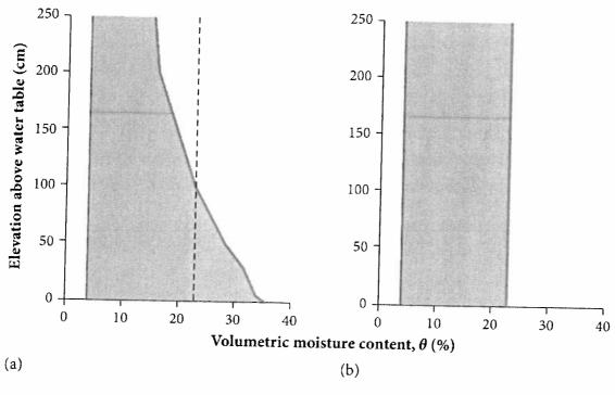
A physical model (a) and an approximation model (b) of the available soil water for plants with a water table at 2.5 m below the land surface – the approximation model uses  $\theta_{pF=2.0} - \theta_{pF=4.2} = 23\% - 4\% = 19\% = 7.6$  cm water for a root depth of 40 cm
