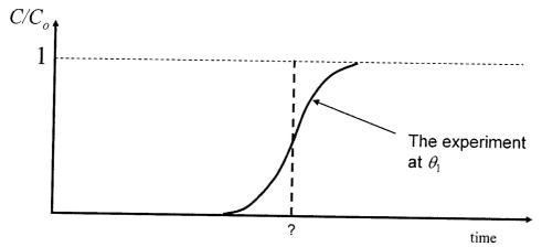
From a breakthrough experiment in a horizontal column of length L the breakthrough curve is recorded. The experiment is performed at soil moisture content  $\theta_1$  and a constant water flux density q. At t=0 a sodium chloride solution (NaCl) is added to the water and the breakthrough curve of the chloride ions  $Cl^-$  is recorded (see the figure above).
