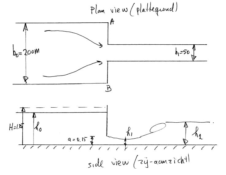
3. A channel with a horizontal bottom has a gate AB at the end with opening  $h_1$ . The velocity head upstream of the gate is measured by a Pitot-tube and is 0.02 m. Given are:
